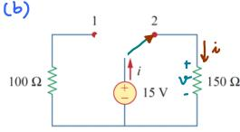
The same reasoning in part (a) also applies to this part except that now the current i is  $15 V = 150 \Omega$  flowing through a new loop in the clock mile direction
