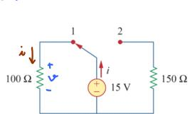
We need to apply Ohm's law. First, note that the is that we draw near the resistor is the same as the is that is coming out of the voltage source. We also add the voltage & across the resistor to use with the Ohm's law. Note that & is connected directly to the 15V source and their polarity matched. Therefore, v=15V.
